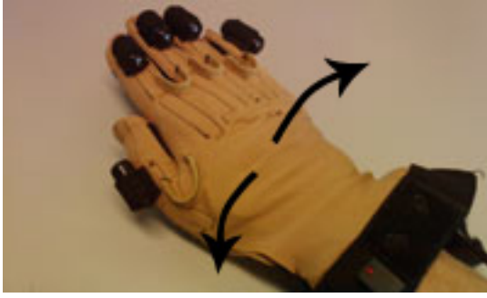
Figure 3: The zoom gesture. Stretching all fingers and pushing them together. Rotating wrist up and down zooms in and out respectively.
